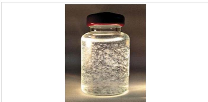
Example of Delamination in Glass Vial (50 ml).
