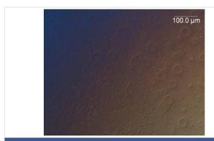
Glass delamination under the Carlton Microscope.
