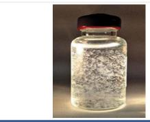
Example of Delamination in Glass Vial (50 ml).
